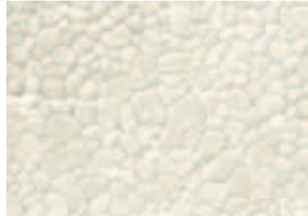
SEM CERCON® microstructure: yttriumoxide stabilized, tetragonal zirconium dioxide (Y-TZP). The fine-grained and dense structure allows the production of implant abutments with high fracture toughness, bending and tensile strength.
